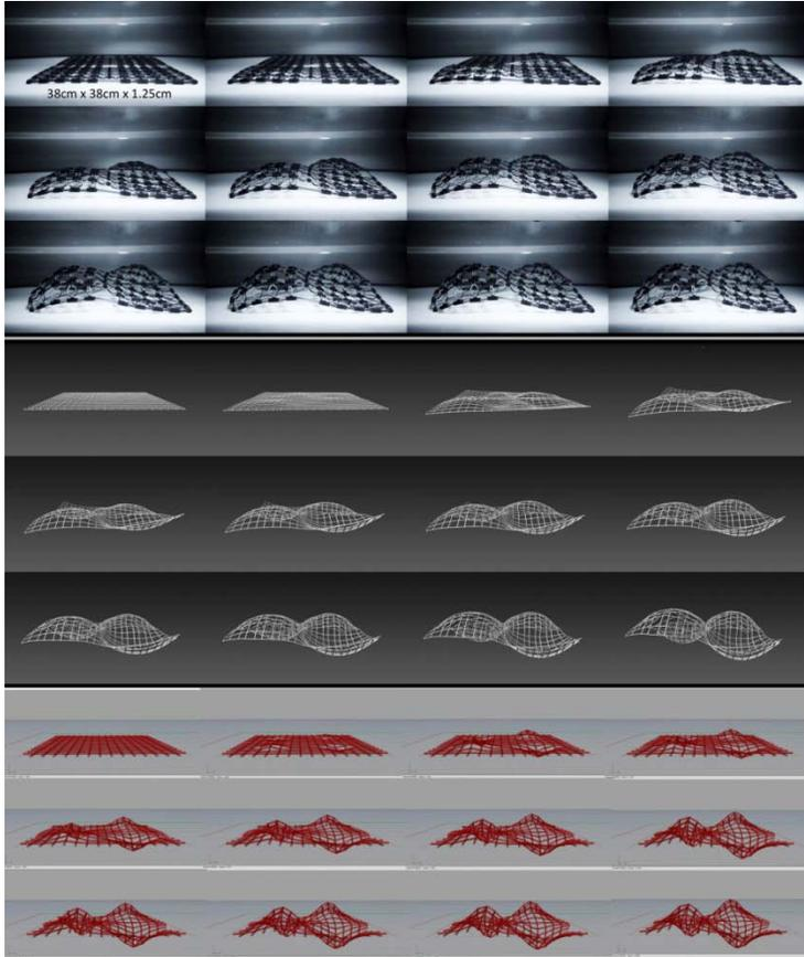
Figure 3. Comparison of two different simulations of the deformation of a 2D grid into a double curvature surface (convex and concave) still-frames sequence (left side one-point perspective) Nelson Montás (2015) based on Raviv et al. (2014). The graphic animations show a strong resemblance between the replication (bottom) and the original model (top) and simulation (middle).
